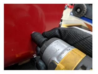
Remove the rear securing bolts at the back of the battery tray. **Tip:** Use a knuckle joint adapter or ball-headed extension in conjunction with a socket in order to get the best possible purchase on the bolt heads.
