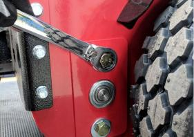
Carefully slide the motor assembly forward within the machine body to release tension in the drive chains.
