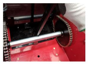
Use an impact wrench to re-tighten the outer bearing mount bolts. If any of the inner nuts fail to 'grab' and instead spin during tightening of the outer bolt, use a long flat-headed screwdriver to hold the nut in place while tightening.
